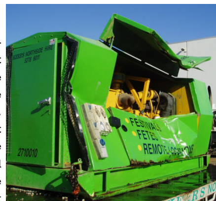
Damage caused when a Front End Loader reversed over this generator.
