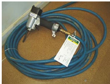
Basso Nail Puncher make light work of the hard job of punching nails down.
