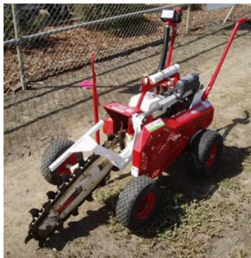
Mini Trencher available in 500mm & 600mm bar lengths 75mm wide.
